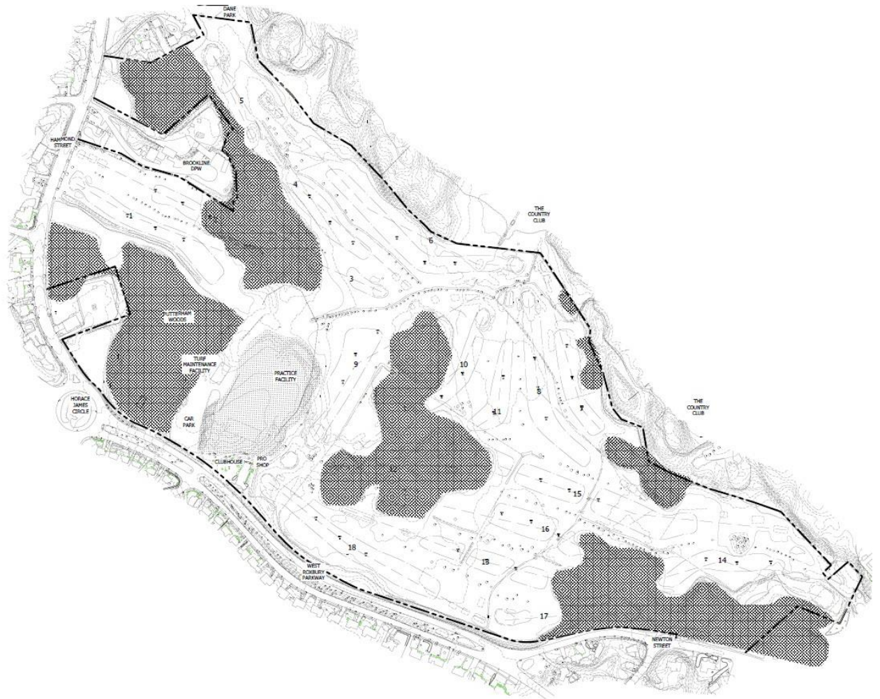
Glacier ledge formations highlighted in dark grey on the property. There is additional ledge under the current driving range, highlighted in a light grey.
