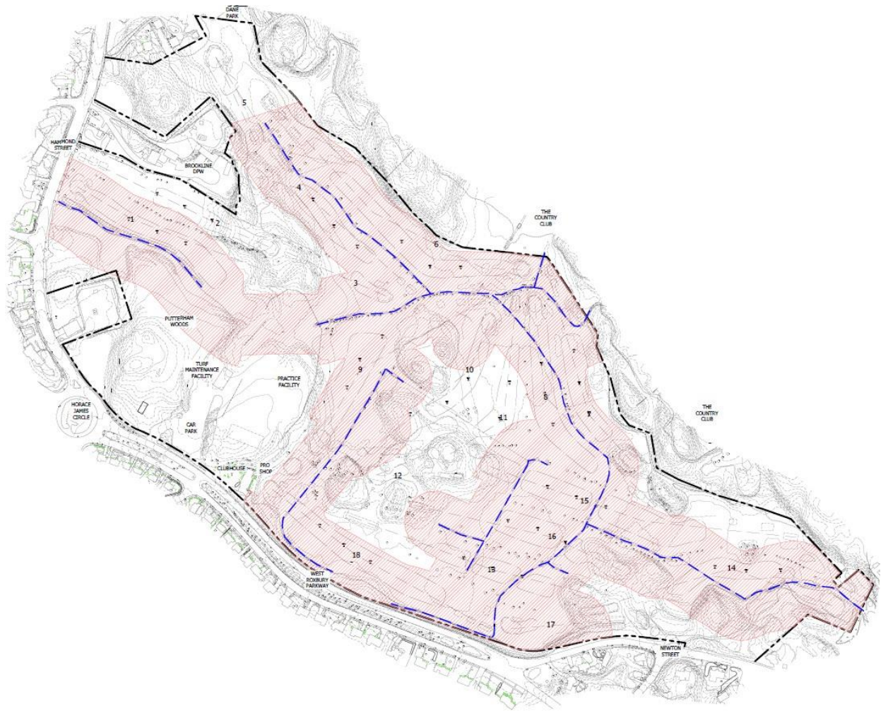
Wetland Jurisdictional Buffer Zones per the Wetlands Protection Act. Areas highlighted in red shading.
